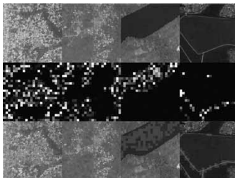
Figure 55.3 Visualization of features. Four different convolutional filters (which identify, from left to right, features corresponding to urban areas, non-urban areas, water, and roads) in the convolutional-neural-network model used for extracting
